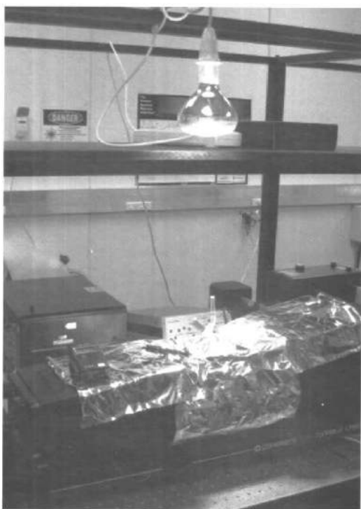
Fig. 3. Heating lamp suspended over a titanium:sapphire laser; the photoacoustic cell is in the laser cavity with its glass tip pointing towards the heat lamp.
