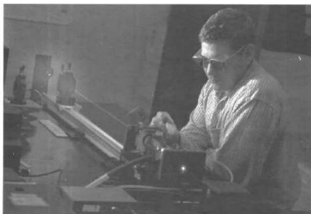
Fig. 2. The dye laser of a photoacoustic spectrometer in operation; the cavity of the laser extends from the bright spot (front) along the visible beam and the sample cell is housed in it.
